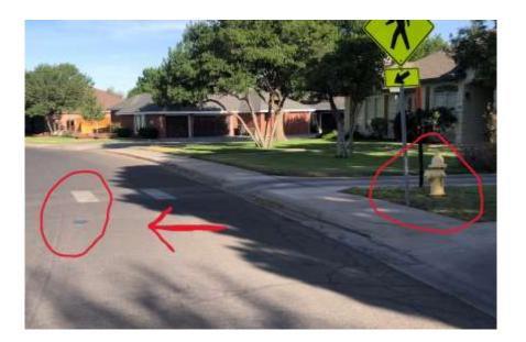
Have you noticed the blue reflective pavement markers being installed on Midland streets? The purpose of these markers is to help emergency personnel locate fire hydrants easily. It is important to be aware as hitting one at the wrong angle or going over a wet one could cause a cyclist to fall.
